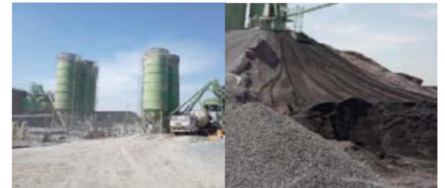
100% Alternate material used. M-Sand and Flyash are used. One Silo out of two are filled with Flyash . So we replace the natural sand with manufactured sand (M-Sand) - AIMS Faridabad
